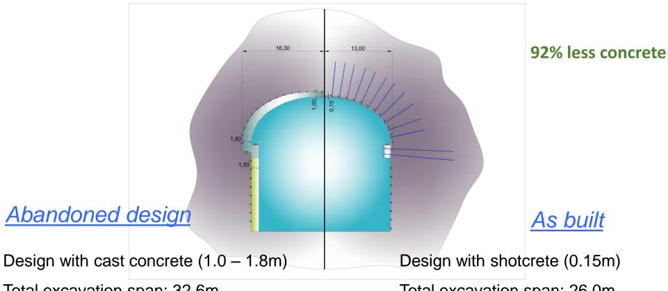
Total excavation span: 32.6m Total excavation span: 26.0m
